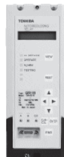
Figure 4. Relay front panel
